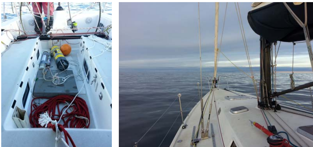
An acoustic data logger (the yellow tube in the cockpit to the left) prepared for deployment not far from Bornholm, on the 45 feet ketch Roxy , December, 2013.
